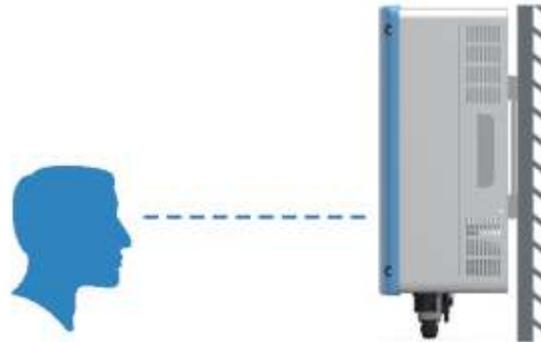
7. The inverter needs to be installed uprightly, and cannot be placed horizontally or upside down, or tilted.
